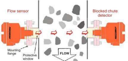
Combining the Microsense blocked chute detector with the Microsense flow switch provides a unique solution for two applications with one installation. For this application we utilise the flow switch on one side of the application and the receiver of the blocked chute switch on the other, as shown in the diagram opposite. This application would detect firstly if there is flow in the chute or pipe and secondly if the chute has blocked.
