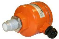
The Microsense microwave switch provides an effective way of detecting the flow or no flow of a wide range of particulate materials. The flow switch uses a microwave Doppler effect and is non-invasive.
