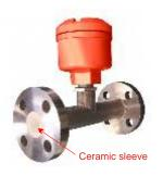
Microwaves will pass through low dielectric materials such as plastic or ceramic, making it possible to monitor in closed pipes. The diagram shows a stainless steel pipe with a sensor process connection half way along. This pipe section also has an inner sleeve made of a durable chemical resistant ceramic. The microwaves from the flow sensor will pass through the ceramic sleeve which is totally enclosed, providing a non-invasive flow solution.
