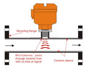
This non-invasive mounting ensures the process remains closed, allowing easy removal of the sensor if required. This drastically reduces wear and tear on the sensor and also allows for easy access to it without having to shut down the process.
